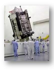
Lockheed Martin's GPS III Non-Flight Satellite Testbed (GNST), a full-sized, functional GPS III satellite prototype, now at Cape Canaveral Air Force Station (CCAFS), Fla., recently communicated via cross-links with Air Force flightlike hardware simulators for the GPS IIR, GPS IIR-M, and GPS IIF satellites, which make up the bulk of the current GPS satellite constellation
